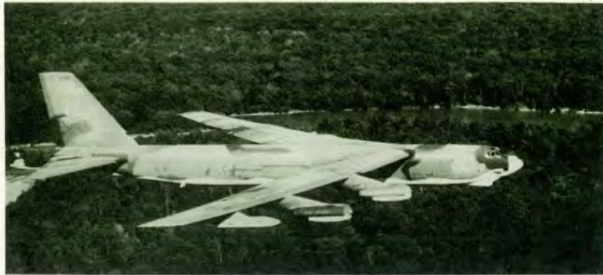
The B-52s that rolled off the assembly line 25 years ago were designed for high altitude bombing missions. To enable them to withstand the severe stresses imposed in low altitude operations, almost all of their load-carrying structure has been replaced or reinforced.
